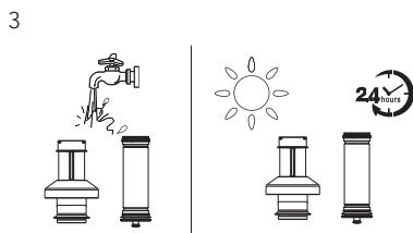
Clean the pre-filter and mesh filter under cold, running water. Air dry completely before reinstalling.
