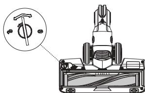
Use a coin or other tool, to unlock the brush roller lock, then remove the brush from the brush window.
