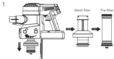
Turn counter-clockwise to remove the filters.
