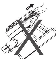
Do not place the appliance as above when removing or installing the HEPA filter, to prevent dust from entering the motor.
