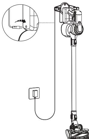
Place the main body on the dock, connect the charging cord to the battery and plug it into the wall outlet. The battery indicator blinking blue indicates that it is charging correctly.
