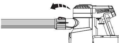
Press the release button to remove the tube.
