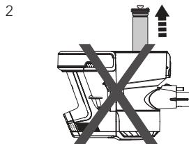
Do not turn the appliance upside down when removing or installing the filter to prevent dust from entering the air channel of the motor.
