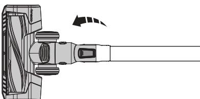
Press the release button to remove the power brush.
