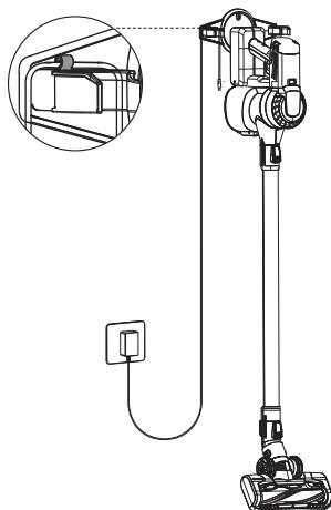
When not charging, stick the power cord into the slot of the dock.
