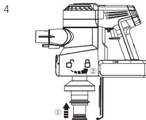
After cleaning, insert the pre-filter into the mesh filter properly and it clicks into place. Install the clean filters back into the main body, then close the dustbin flap.
