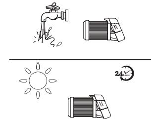
The HEPA filter can be washed under running water and must be completely dry before reinstalling.
