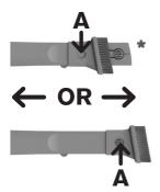
2-IN-1 COMBO TOOL: Use the Crevice Tool for tight spaces, corners and along stair edges and baseboards. Try the Dusting Brush for furniture, table tops, lamps, blinds and more.Press the lock button (A) down and slide to switch between modes. EXTENSION WAND: Attach to cleaning wand for longer reach on above
