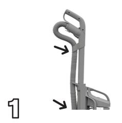
INSERT CLEANING WAND INTO TOP OF VAC. SECURE YOUR HOSE HERE AND HERE.
