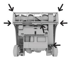
3. Slip belt around the brushroll in area without bristles (A) and metal pin (B). Each end of the brushroll will fit into pockets on each side of the nozzle (C). Put the plate back on and screw together. 2. Then take off that old belt. Slide on a new belt with the lettering on the outside.
