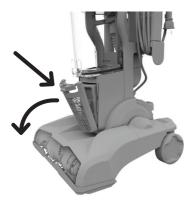
3. Put the dry filter back. Now line up the filter cover with the bottom tabs first and then snap back into place.
