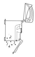
1 Empty dust cup when debris reaches MAX fill line. Remove by pulling up on latches on dust cup handle.
