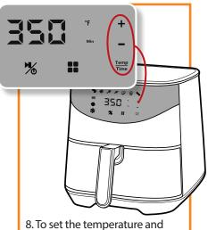
8. To set the temperature and time manually, or to adjust the preset temperature or time, tap the +/- icons. Tap Temp/Time to alternate between setting temperature and time.
